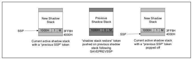
Figure 17-3. SAVEPREVSSP to Save a Restore Point
