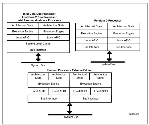
Figure 2-6. Intel 64 and IA-32 Processors that Support Dual-Core
