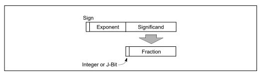
Figure 4-11. Binary Floating-Point Format
