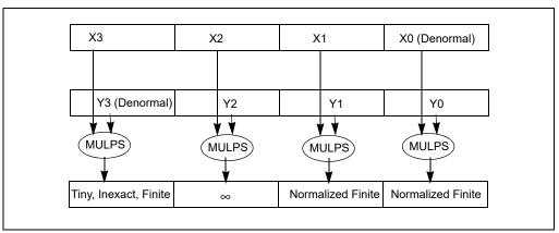
Figure 11-9. Example Masked Response for Packed Operations
