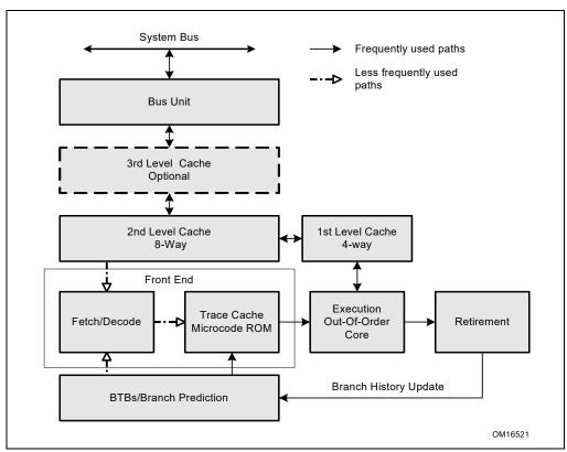
Figure 2-2. The Intel NetBurst® Microarchitecture
