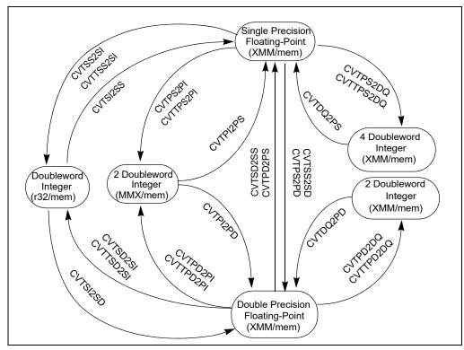
Figure 11-8. Intel<sup>®</sup> SSE and SSE2 Conversion Instructions
