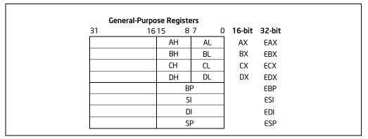
Figure 3-5. Alternate General-Purpose Register Names
