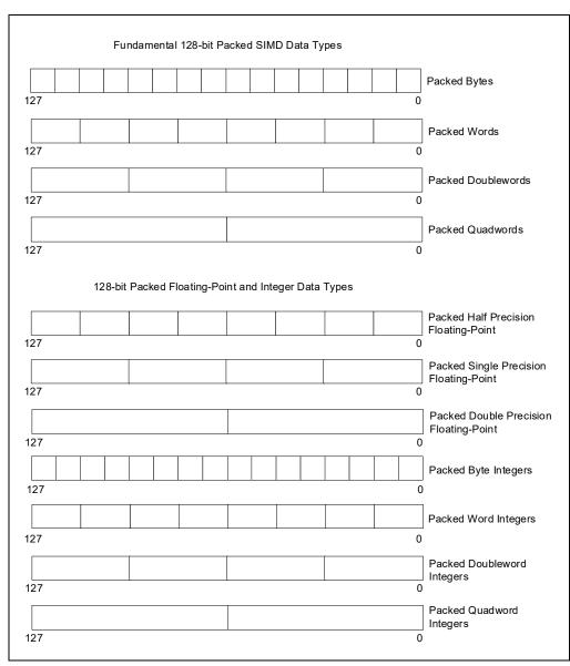
Figure 4-8. 128-Bit Packed SIMD Data Types
