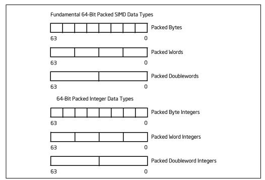
Figure 4-7. 64-Bit Packed SIMD Data Types
