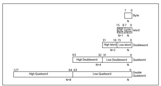
Figure 4-1. Fundamental Data Types
