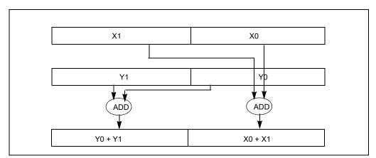
Figure 12-2. Horizontal Data Movement in HADDPD
