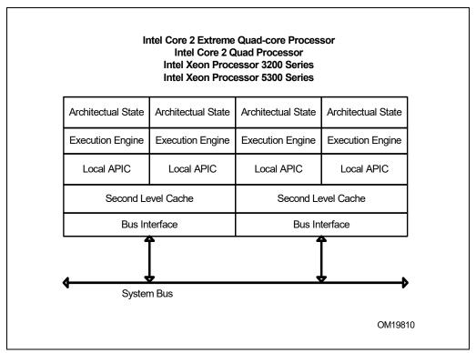
Figure 2-7. Intel<sup>®</sup> 64 Processors that Support Quad-Core
